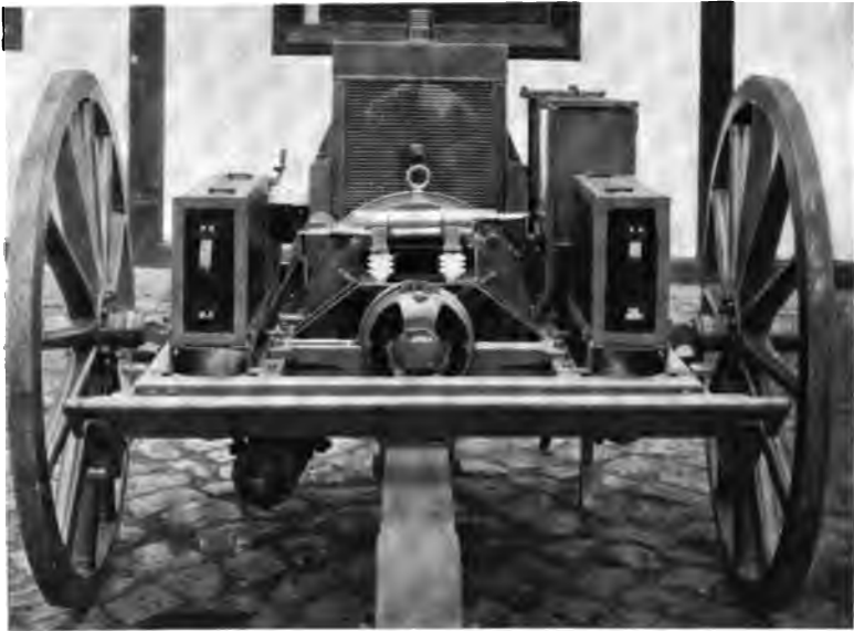
a. Generating plant wagon (alternator side).
